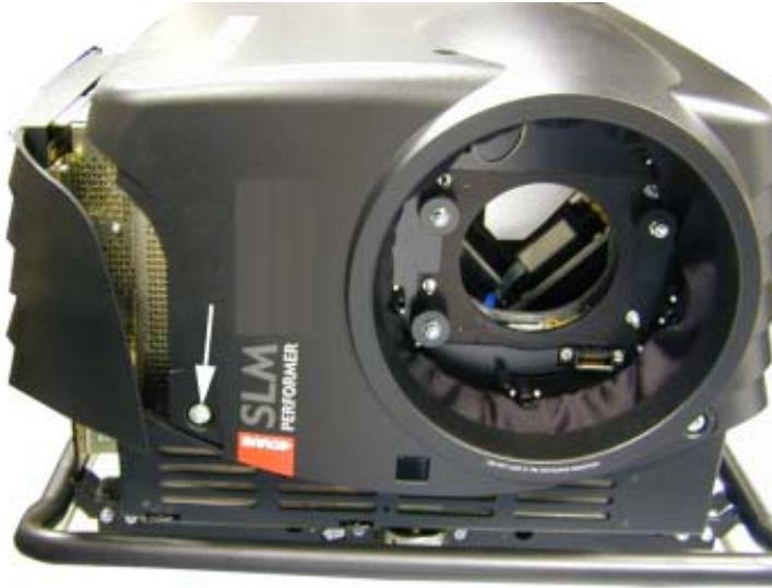
Image B-3 Front screw top cover removal
